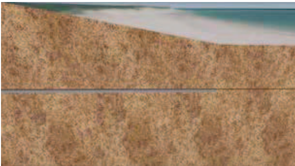
3. Pilot bore exits at reception pit
